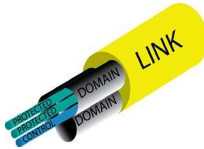
Figure 42: With multiple VLANs on a link one is a control VLAN with protects the other VLAN
